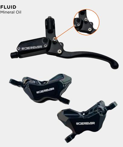
For tricycles, duo calipers with excellent braking force.
